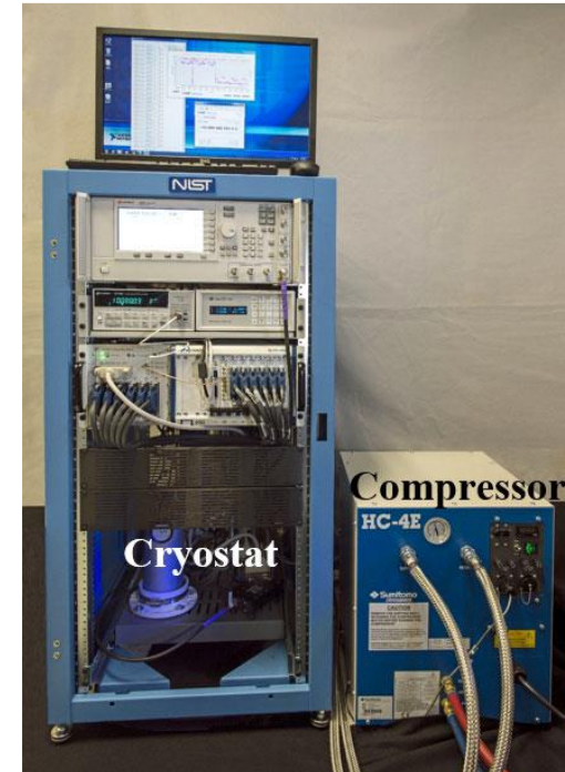
NIST SRI 6000 Programmable Josephson Voltage Standard (PJVS)
